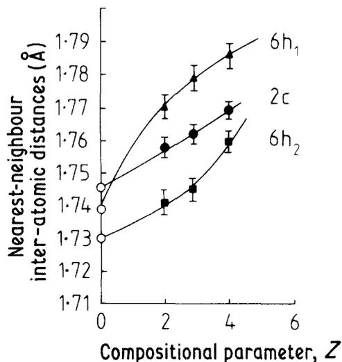
Figure 3 Compositional variations of the (Si, Al)  $\rightarrow$  (O, N) nearest-neighbour inter-atomic distances for  $\text{Si}_{6-Z}\text{Al}_Z\text{O}_ZN_{8-Z}$  obtained using the profile refinement method.
