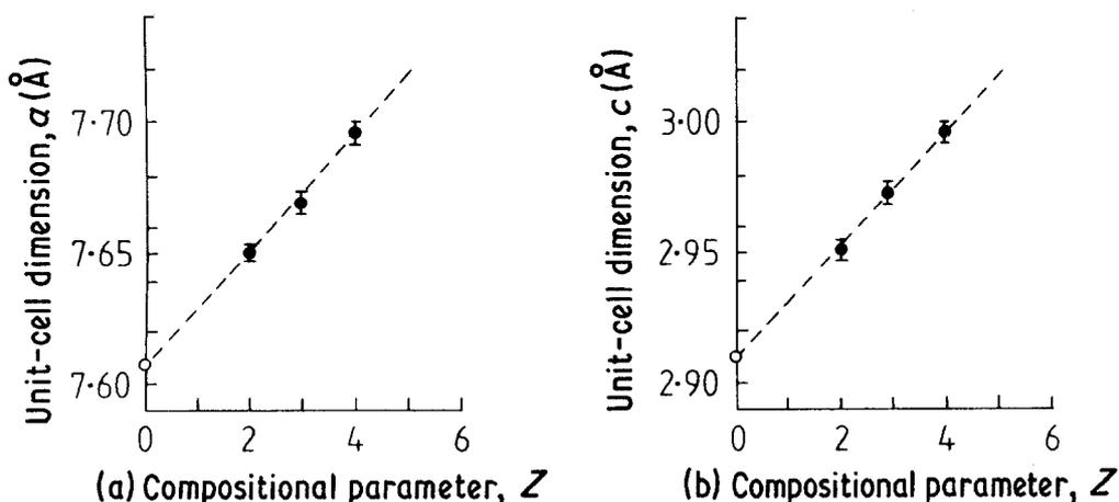
Figure 2 Compositional variations of the unit-cell dimensions (a)  $a$  and (b)  $c$  for  $Si_{6-Z}Al_ZO_ZN_{8-Z}$  obtained using the profile refinement method.
