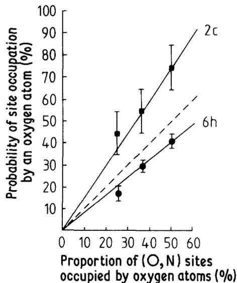
Figure 4 Probability of site occupation by an oxygen atom plotted against the percentage of oxygen atoms among the (O, N) atoms for  $\text{Si}_{6-Z}\text{Al}_Z\text{O}_ZN_{8-Z}$  obtained using the profile refinement method.
