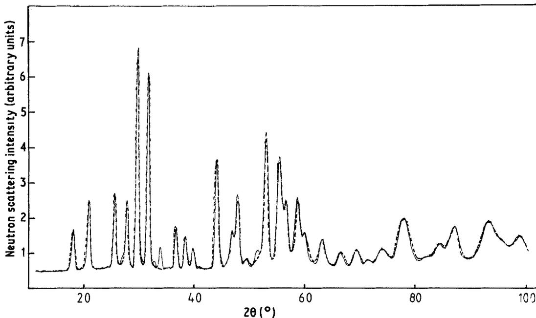
Figure 1 The neutron diffraction pattern of the  $\beta'$ -sialon  $\text{Si}_2\text{Al}_4\text{O}_4\text{N}_4$  measured at 4.2 K. Continuous line: experimental data; broken line: the fitted profile, with a reliability factor of  $R = 9.3\%$ .
